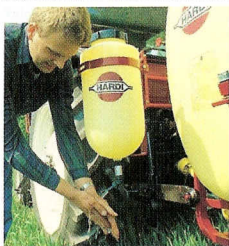
15 l Clean water tank
